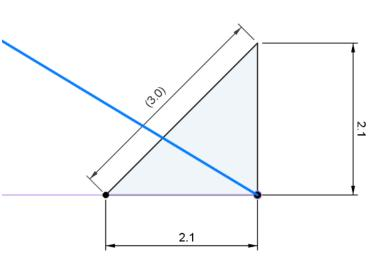
Here you are going to place the 2 flags before the finish. Take one tape measure to the 8.5m mark on the ground and go up 4.6m. Then take another tape measure from the 4.6m mark on the perpendicular tape and go out to meet 8.5m tape. Repeat this for the second flag on the 10.4m mark. From the 13.4m mark go up 10.4m, then from the 10.4m mark go out 13.4m. Place a flag holder where each intersects.
