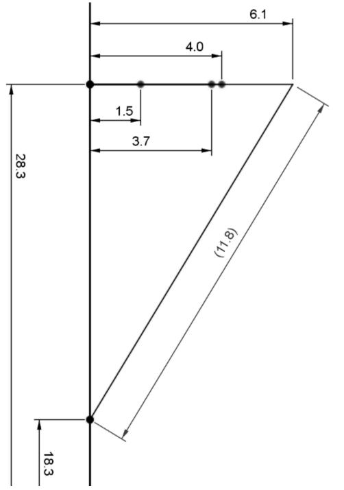
Now go back to the 18.3m marker and walk out 31.3m. From the 35.4m marker walk out 26.2m. Where these two tapes meet pound a gate rebar. Also pound a gate rebar at 24.1m. At the 23.5m mark, pound a flag stake. This MUST be a stand alone flag, not on a flag on a gate!
