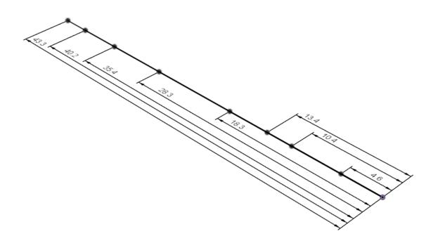
Go to the 13.4m mark and extend the tape measure out 26m. Extend another tape measure from the origin 22.3m. Pound a rebar for a gate. Also place markers at 13.4m and 8.5m.
